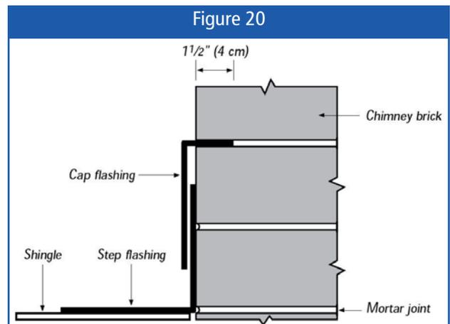
joint with mortar or Asphalt Plastic Cement. Finally, bend the flashing down to cover the base flashing and to lie snugly against the masonry. Don't fasten through the base flashing, as the two must be allowed to move independently.
