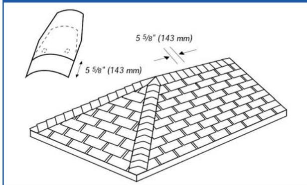
Nail cap with one nail on each side 15,2 cm (6") from the exposed end and 2,5 cm (1") from each side. The same method applies for the hip and ridges.
