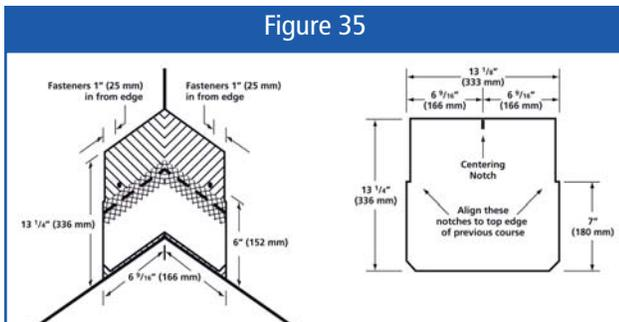
All subsequent rows are formed by bending the hip and ridge shingle along the centerline leaving a 14.3cm (5 5/8") exposure (see **Figure 36**).
