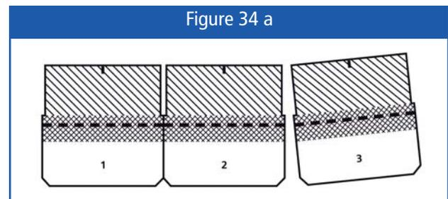
be installed as a single layer hip and ridge or the tabs can be superimposed to form a double layer Hip and Ridge.
