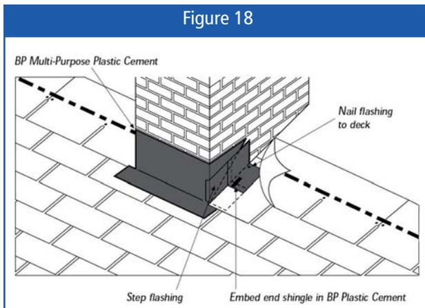
vertical wall. Cut, bend and apply the step flashing as shown in Figure 18 and as described in Section 3.6-A. Secure each flashing unit to the deck with nails. Embed the end shingles in each course that overlaps the flashing in Asphalt Plastic Cement.
