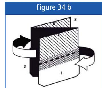
Hip application starts at the eave end of the hip and works up to the ridge. Application of the ridge on a hipped roof starts at each end and meets in the middle. Application of ridge on a structure with no hips starts at the end opposite to prevailing winds and continues to the other end.
