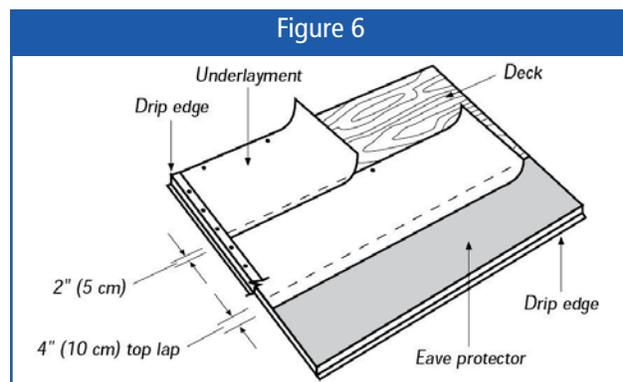
Nail sufficiently to hold the underlayment in place until the shingles are applied. Install shingles as soon as possible after installation of the underlayment. Building Products of Canada Corp. recommends installing the shingles the same day as the underlayment, to keep
