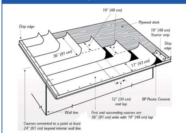
line. Beyond this point 91 cm (36"), sheets are laid, but without Asphalt Plastic Cement, lapping each course 48 cm (19") over the preceding one. Each course of felt is nailed sufficiently to hold it in place until the shingles are applied (see Figure 9).
