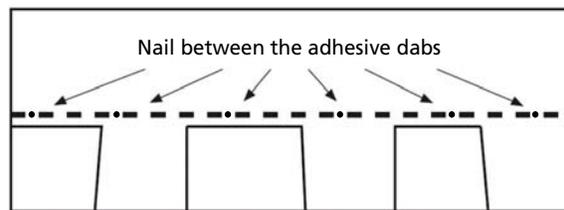
shingles must be fastened using 6 nails and all shingles located at the roof edges must be cement together in a 10 cm (4") wide layer of plastic cement. If above special application instructions are not followed, shingles will be warranted for winds from 115 km/h (70 mph) to 180 km/h (110 mph). See Table 1 for High Wind Warranty wind speed for the shingle being installed.
