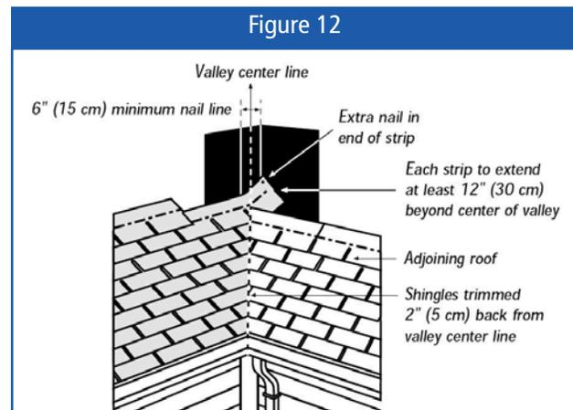
Installing a layer of GRIPGARD, GRIPGARD SX or PROGARD ULTRA Waterproofing Membrane in the valley, instead of roll roofing will ensure maximum protection.
