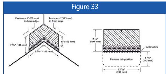
Meridian 3D Hip and Ridge shingles are packaged as pre-scored shingles that separate in three slabs without having to use a knife (see Figure 34 a). Meridian 3D can
