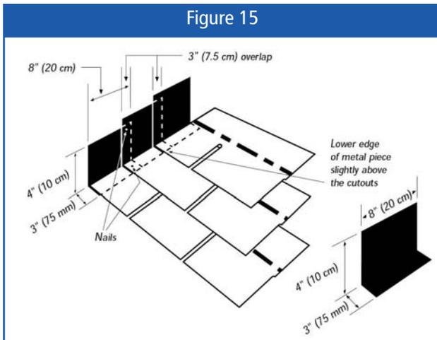
In re-roofing (application over an existing layer of shingles), ensure that the old shingles butting the wall are in good condition. Apply a strip of BP Smooth Surface Roll Roofing 20 cm (8") wide over the shingles along the wall. Nail 10 cm (4") apart along each edge of the strip. Cover with Asphalt Plastic Cement and embed the new shingles. Use a caulking gun and draw a bead of Asphalt Plastic Cement between the ends of the shingles and the siding.
